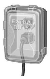
2.20.2 GFCI **NO GFCI**  It is recommended that GFI protected receptacles be installed within 6 feet of any water sources as well as receptacles found outside below 2.5 meters. It is recommended to have a qualified electrician install these.
